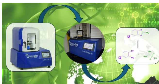
Figure 1. 2-Amino-benzoxazole synthesis through the use of Resonant Acoustic Mixing (RAM).
